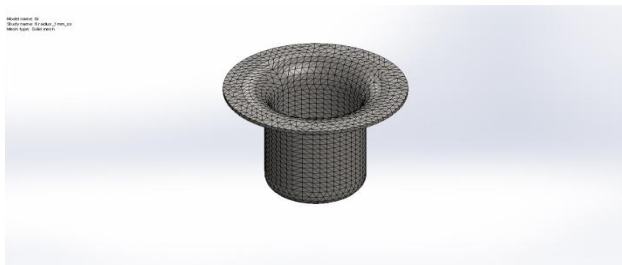
Fig 4(a): Stainless Steel cup meshed model
